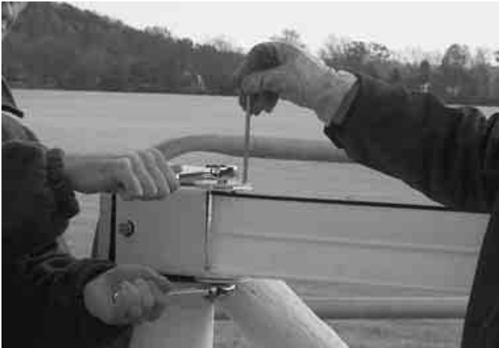
Photo A.6 Tightening the rail.
