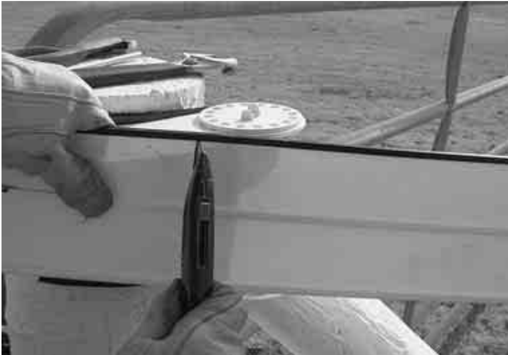
Photo A.4 Cutting the Rail to length.
